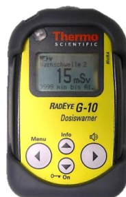
Abbildung 40: Dosiswarner Thermo Fisher Scientific RadEye G-10
